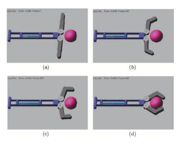
Figure 5. Simulation results for capturing an object.
