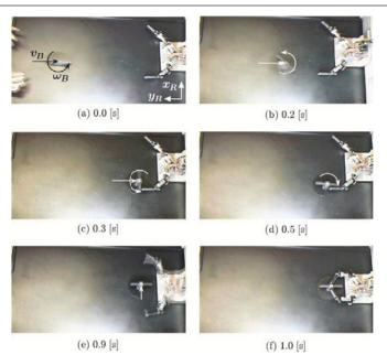
Figure 7. Two-fingered hand captures an object by 2-step strategy.
