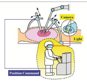
Figure 12. An example of medical robot system.
