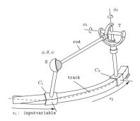
Figure 5. The concept of a spline joint and its use in kinematical loops.
